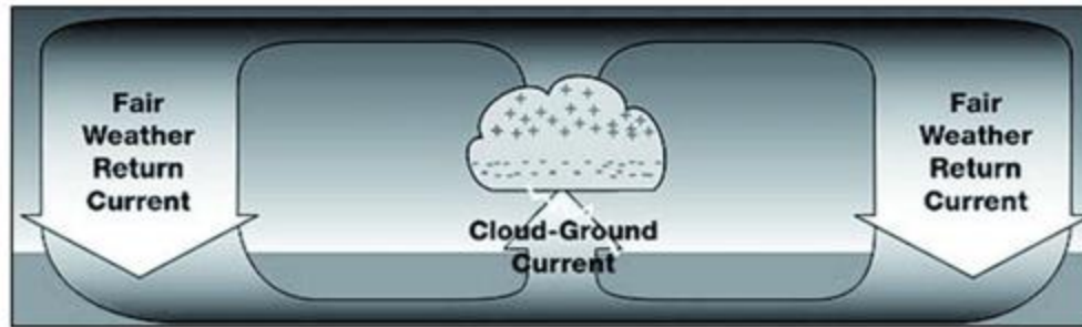
Figure B-1. Global electrical circuit. A current coming up from the ground at the location of lightning (depositing electrons into the earth) and returning to the ground elsewhere. Source: NASA/MSFC (Dooling)
