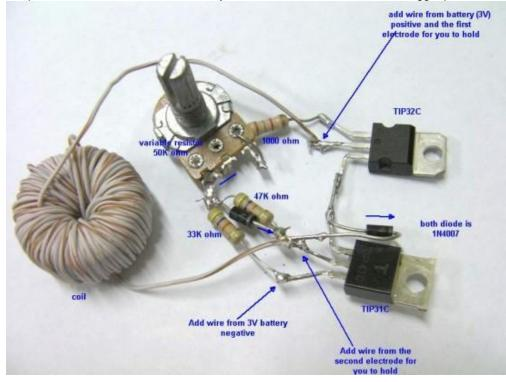
The photo below illustrate the correct way to connect the transistor, click for bigger picture:
