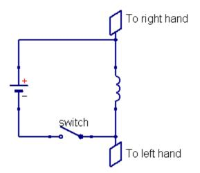
The power of this zapping method is proportional to the source voltage and the inverse of the coil resistance. Using a 1.5 volt battery and coil with 1 ohm resistance, you may not feel anything, but the same coil with 12V power source will produce very sharp or painfull zap.
