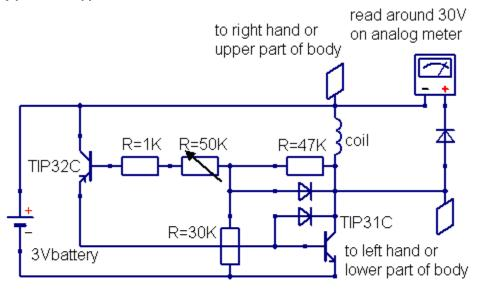
I call it stingo zapper. The coil use ferrite toroid core. The variable resistor will allow you to change the power level and the frequency. To limit the output power to increase safety, it use two 1.5V battery as power source. At minimum power it can make people sleepy, at high power level you can feel painfull zapping. You don't need to use painfull power level, you will see results even if you set this at pain less setting.
