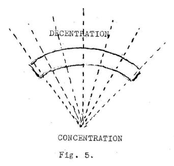
Fig. 5 represents concentration of light rays to a point. Light rays thus concentrated through a lens will burn a hole through paper or fabrics.
