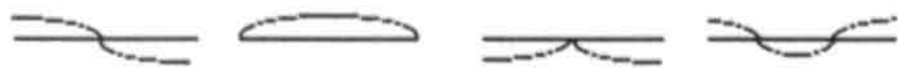
Modes developing in a vibrating flat metal plate.
