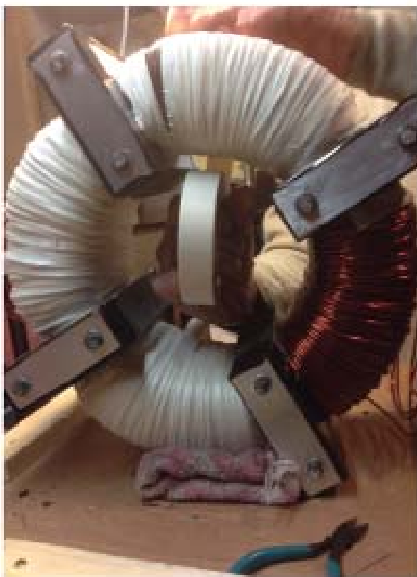
Installing outer wrap on core
